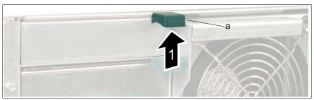
Figure 45: Unlocking the handle
